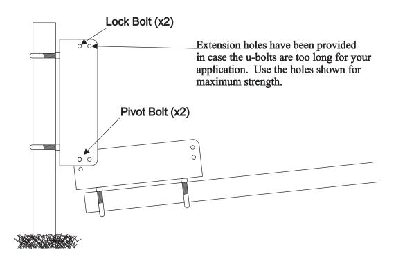
Base Support: Your base support pipe (not included with the MFJ-1903 kit) should be made from thick-wall steel or aluminum tubing and extend at least 3 to 4 feet below ground. For multi-band verticals, we recommend seating the pipe in a 10-inch diameter posthole filled with ready-mix concrete to ensure stability. Note that antenna base supports should always be located well clear of power lines or neighboring property to avoid exposure to life-threatening injury or liability.
